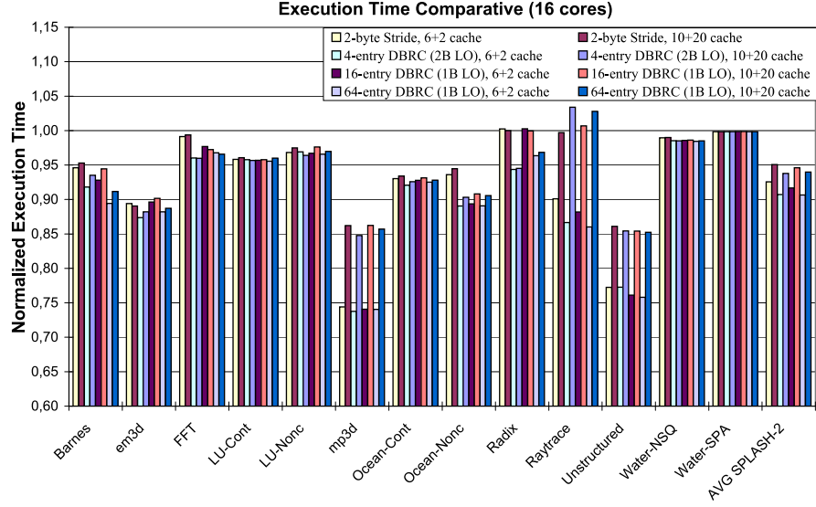
Figure 4.9: Normalized execution time when heterogeneous links are used for different L2 cache access time parameters.
