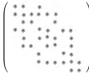
Figure 8.4 Stiffness matrix induced by the discretization of Fig. 8.3
