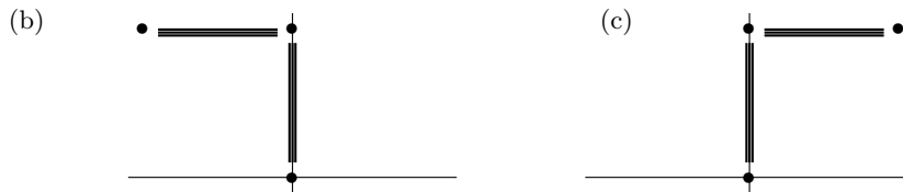
Figure 2.5 Difference stencils of the implicit discretizations (3.31)
