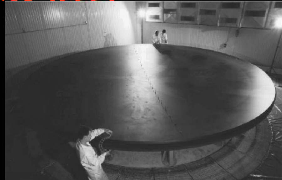
Figure 2 - VLT Primary mirror blank in production (courtesy SCHOTT)
