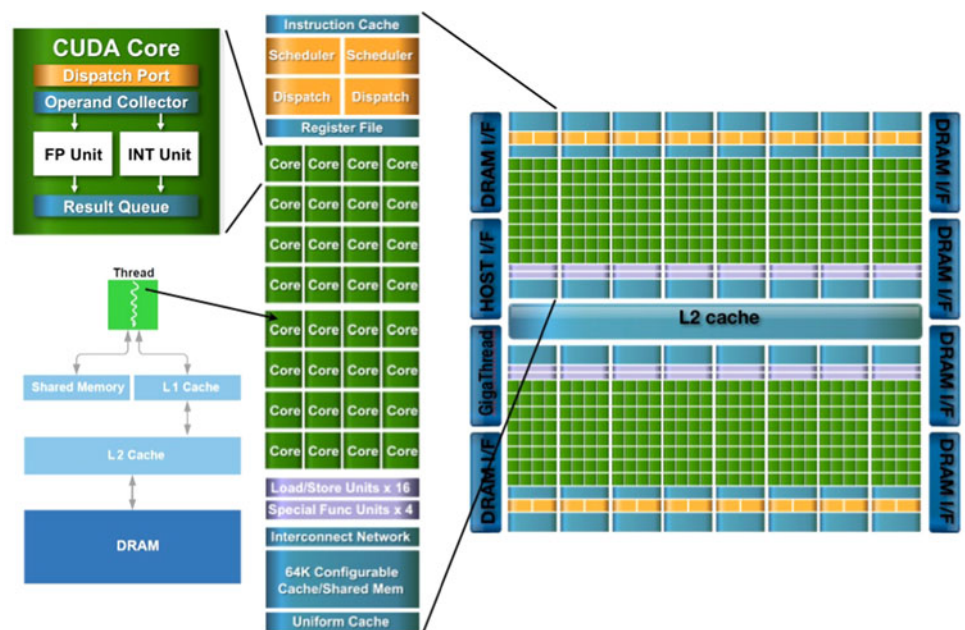
Fig. 5 An outline of the Fermi architecture used within the Tesla M2050 GPU. We have 16 multiprocessors, each composed of 32 cores. An L1 cache (up to 48 KB) is introduced in parallel to the shared memory, and even an L2 cache emerges with 768 KB. More resources are devoted to floating-point arithmetic too
