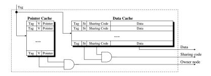
Fig. 1. Organization of the L2 caches required by Direct Coherence.
