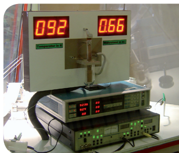
Measuring the critical temperature and resistance of a superconductor in Graz, Austria. Photo courtesy of Simplicatus
