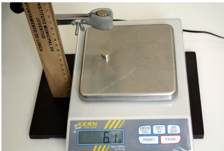
Figure 2.- Measuring the repulsive force between two magnets with an scale.
