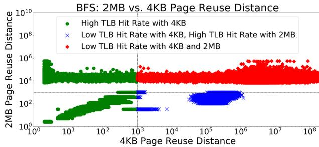
**Figure 2: Characterization of data accessed based on page reuse distance with 2MB vs. 4KB pages, running BFS on a Kronecker network. *HUBs* (blue) have low TLB hit rates with 4KB pages, but high TLB hit rates with 2MB.**
