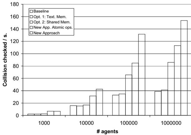
Figure 11: Collisions rate on Tesla C1060 card
