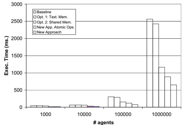
Figure 9: Execution times on Tesla C1060 card
