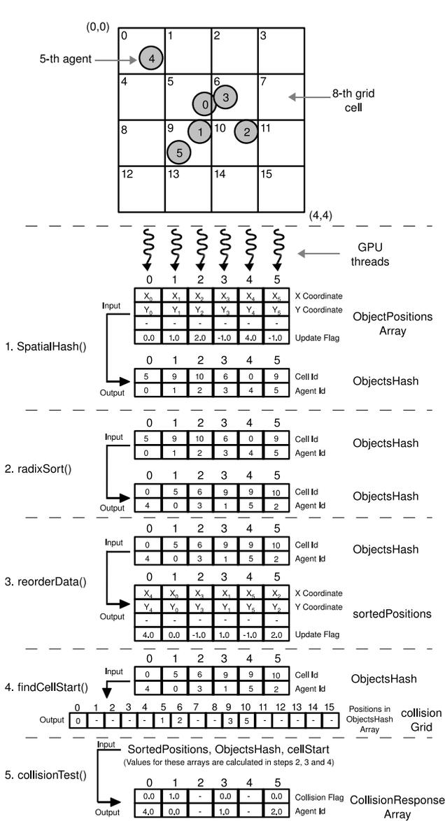
Figure 2: Baseline algorithm for GPU-based collision check
