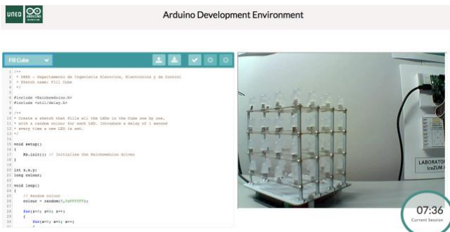
Fig.5 GUI of the 3D LED cube experiment in the Arduino remote laboratory.
