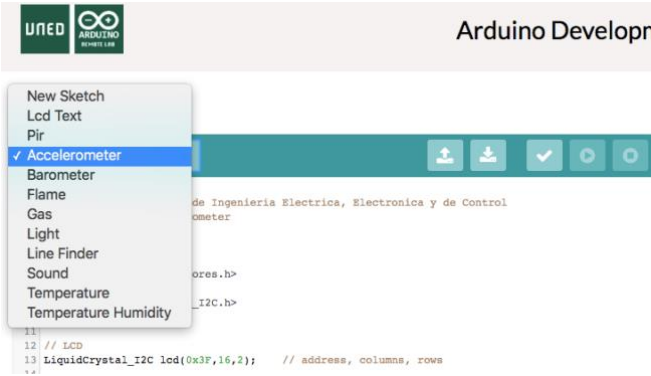
Fig.3 Details of the drop down menu with code examples for the sensors lab that are ready to be loaded in the editor
