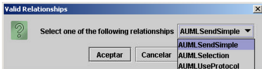
Figure 39. Dialog window for determining the type of connection between two lifelines
