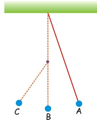
$$T = 2(t_{AB} + t_{BC}) = 2\left(\frac{2\pi}{4}\sqrt{\frac{L}{g}} + \frac{2\pi}{4}\sqrt{\frac{L}{2g}}\right) .$$
